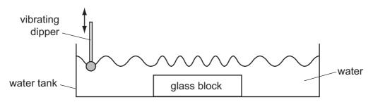
What happens to the frequency and to the speed of the wave as it reaches the glass block?
